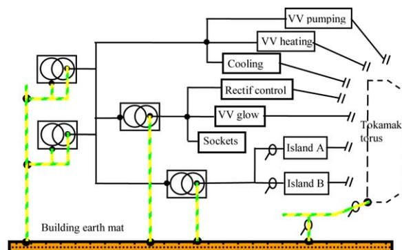
Fig. 2. Earthing scheme in the TCV tokamak hall.
