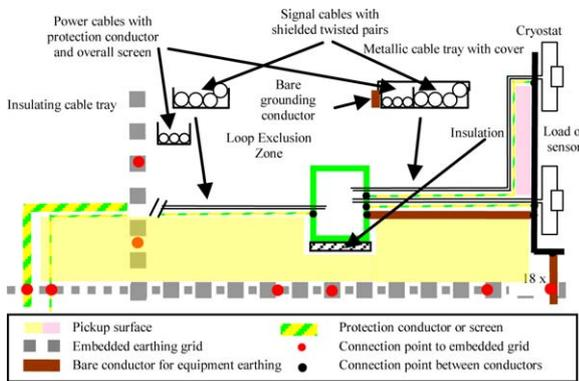
Fig. 4. Earthing concept in the ITER tokamak hall.
