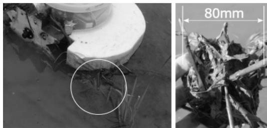
**Fig. 7.** Example of the accident in Case 1-2 (left) and the causal obstacle (right).
