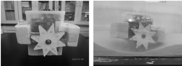
**Fig. 10.** Experimental robot (left) and its traveling test in the water tank (right).
